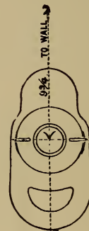
Diagram showing Base of Bowl and giving the closest measurement at which Bowl can be set.
